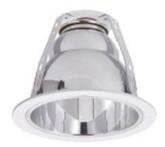
Description : Steel body & trim / Aluminum reflector. Sand white powder coating. Shiny reflector. Fixed downlight. Suitable for recessed T-bar or concealed ceiling. Available in white.
